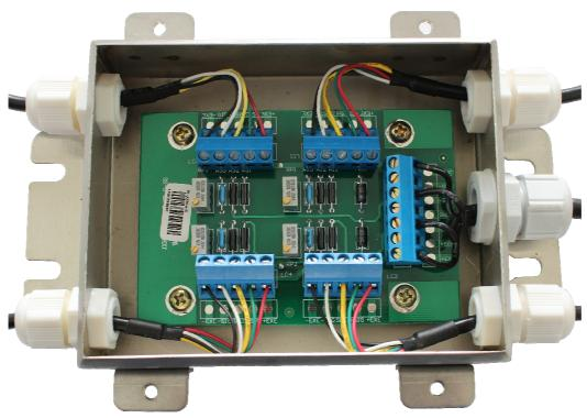
Ensure a careful routing of the cables. The junction box should be mounted in a dry, protected place.
