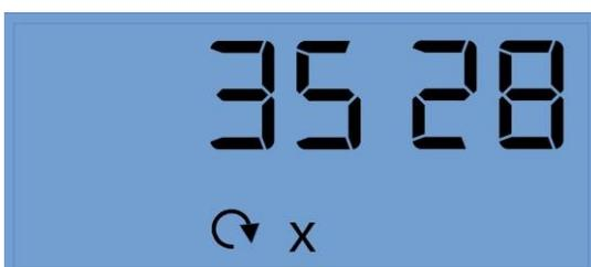
The sum of the counted revolutions is displayed, the symbol with the rotary arrow and the x light up.
