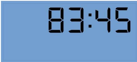
If the colon is visible as a separator, it is hours and minutes.
