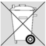
Dispose of the device as part of the final shutdown or parts of it environmentally friendly and sorted (metal to the respective metal scrap, plastic to the plastic waste, etc. - do not dispose as household waste)!
