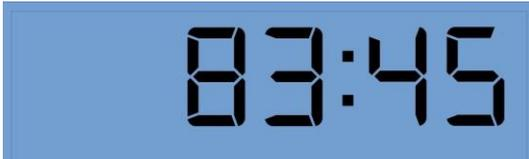
If the colon is visible as a separator, it is hours and minutes.
