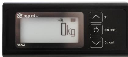
As a practical example, take a pallet with 1000 kg, in which the indicator shows, for example, 1200 kg before calibration. The displayed value of the actual load can be adjusted with the calibration process described above.
